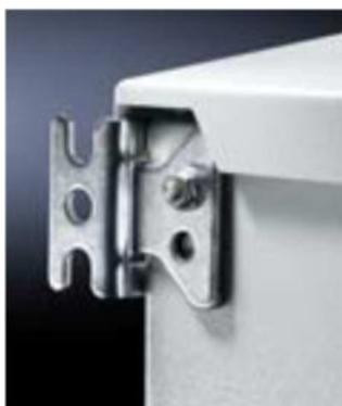
For fast, time saving installation of the indicator box, use wall mounting brackets. Simply insert the expandable dowel into the hole on the backside of the box from the outside and screw-fasten the wall bracket from the outside. In this way the wall bracket securely can be tightened without opening the box door.
