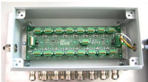
Fig. 10: Terminal box opened
